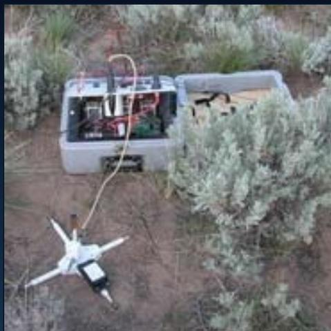
Integrated electric and magnetic field sensor for subsurface mapping in field use.
